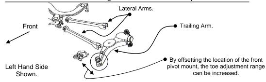
SPF2536K - Rear Trailing Arm Front Bush Kit (*Replaces OEM Part No 1J0505171B*) Fits All Wheel Drive variations of the VAG A4 Chassis as used on the following models:
