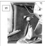
Re-fit front scuttle panels and under dash shelf/ glovebox assemblies. (Mk1 shown)
