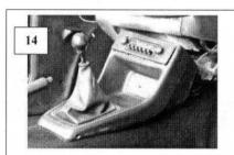
Re-fit the centre console as necessary & gear knob.
