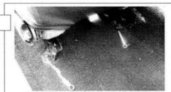
Mk2 - Undo seat bolts & remove front seats.
