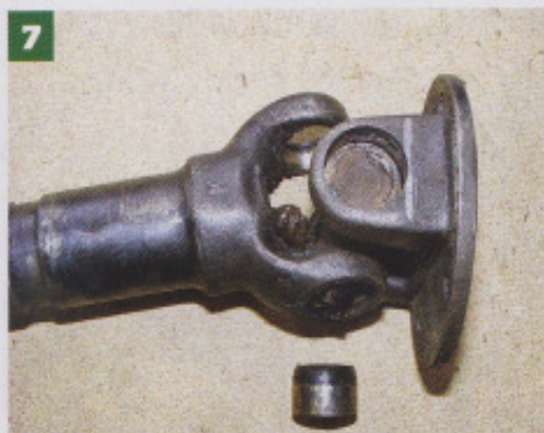
7 The spider can now be tilted and the opposite cup removed. This then allows the two yokes to be separated. Repeat the process to remove the joint completely.
