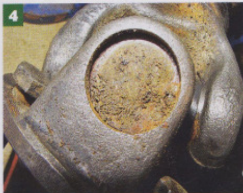
4 The joint should now look like this. Next, find two sockets or similar tubular items, one of a slightly lesser diameter than the cup and another greater.
