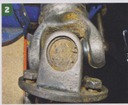
2 Each bearing cup is retained by an internal circlip. These may be rather dirty or rusted, so give them a soak in some release fluid before attempting to remove them.
