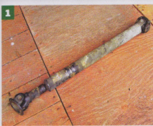
1 Remove the propshaft. This is the general state of most hard-worked driveshafts. An opposite twist of the flanges often reveals a little play in the universal joint's bearings.
