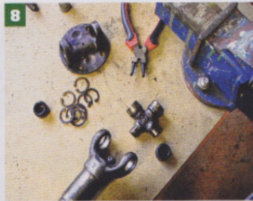
8 The result should be a bunch of components looking something like the above. Repeat the process for the opposite end of the propshaft and clean up the remaining areas ready for paint.
